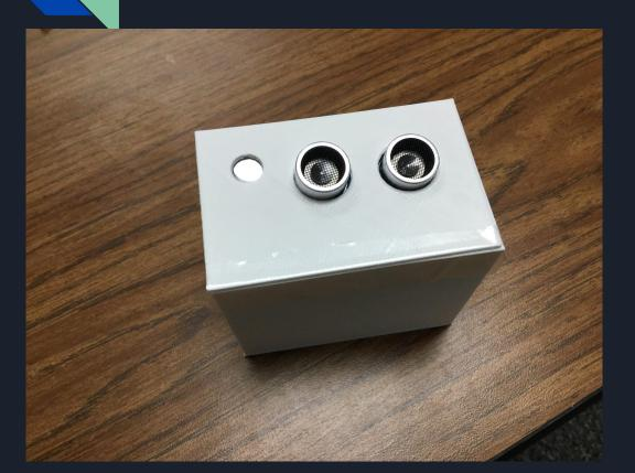
This is the beta version of the Steek. It will detect obstacles and give a warning when the obstacle gets close. It can be programmed to fit the desired distance of the user.
